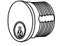
Cylinder 1-5/32 in Diameter hole x 1 in Depth. 5-PIN Schlage "C" Key Way (will not sit flush with door)
