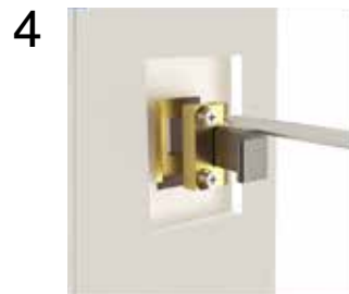
4 Reattach bolt Slightly rotate loose thumb turn to make lock body screws visible Reinstall bolt assembly by aligning screw holes Tighten screws Use thumb turn to fit bolt assembly back in
