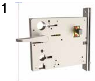
1 Expose screws Rotate thumb turn 90 degrees to project bolt and expose the two bolt screws
