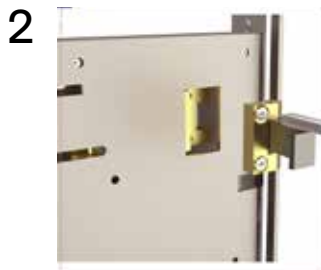
2 Remove bolt from lock body Extend the bolt and loosen screws without removing them and remove bolt assembly from the lock
