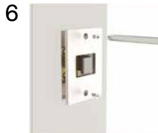
6 Mount cuff Mount the bolt cuff aligning per template Install trim accordingly
