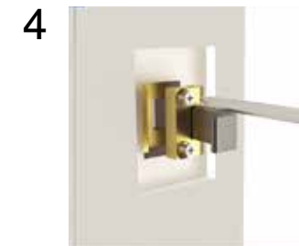
4 Reattach bolt Slightly rotate loose thumb turn to make lock body screws visible Reinstall bolt assembly by aligning screw holes Tighten screws Use thumb turn to fit bolt assembly back in
