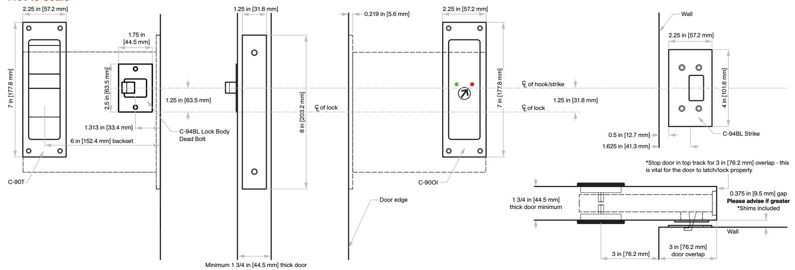
**Note:** Door size = opening width plus 6 in [152.4 mm] Example: 40 in [1016 mm] opening + 6 in [152.4 mm] = 46 in [1168.4 mm] wide door
