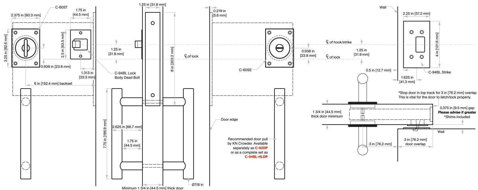
**Note:** Door size = opening width plus 6 in [152.4 mm] Example: 40 in [1016 mm] opening + 6 in [152.4 mm] = 46 in [1168.4 mm] wide door
