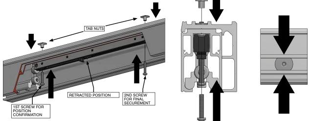
NOTE: ENSURE AREA OF TRACK WHERE CATCH 'N' CLOSE DEVICE WILL BE INSTALLED IS FREE OF FASTENERS. SECURING CATCH 'N' CLOSE DEVICE ONTOP OF A FASTENER MAY LEAD TO OPERATION ISSUES OR DAMAGE TO THE SYSTEM.
