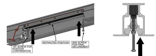
NOTE: ENSURE AREA OF TRACK WHERE CATCH 'N' CLOSE DEVICE WILL BE INSTALLED IS FREE OF FASTENERS. SECURING CATCH 'N' CLOSE DEVICE ONTOP OF A FASTENER MAY LEAD TO OPERATION ISSUES OR DAMAGE TO THE SYSTEM.
