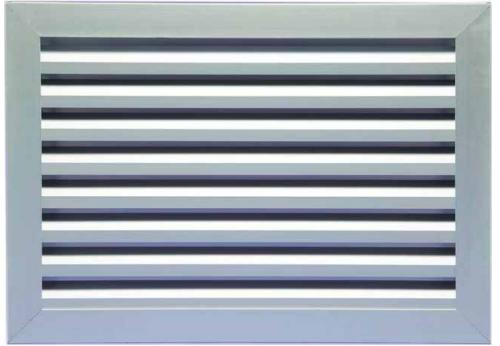
CDL with inverted "Y" blades are easy to install, attractive in design and are suitable for plastic laminated, wood and hollow metal doors. Other features include aluminum's acceptance to a wide range of finishes; resistance to loosening of screws due to vibration by having frame sections clamped together by unique, durable nylon clip. Free area of approximately 30%.
