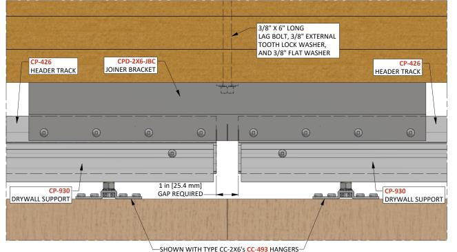
3/8" X 6" LONG LAG BOLT, 3/8" EXTERNAL TOOTH LOCK WASHER, AND 3/8" FLAT WASHER CPD-2X6-JBC JOINER BRACKET CP-426
